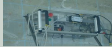
surface wave air coupling
